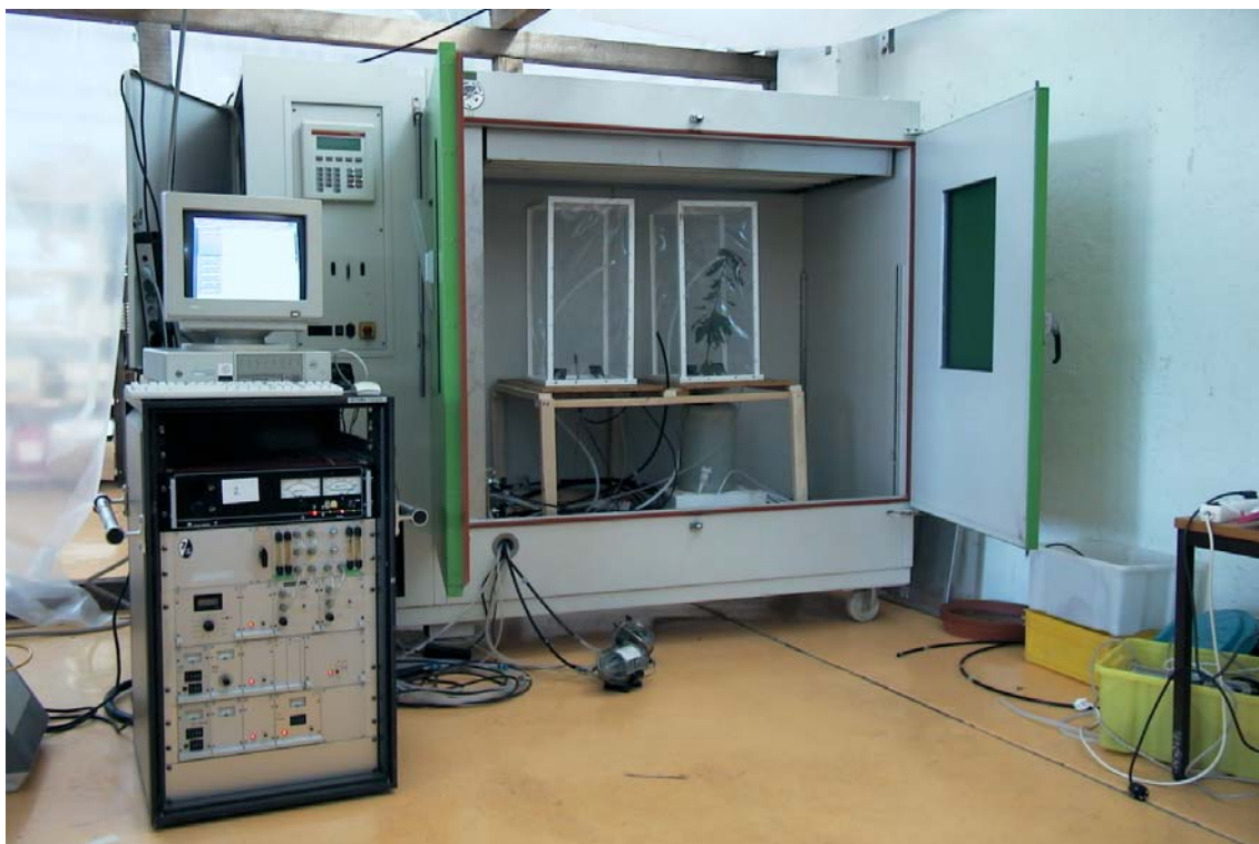
Fig. 1. Chamber system used for the analysis of the reactive atmospheric trace gas acetaldehyde.
